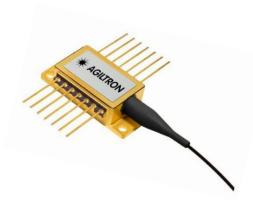
The 830nm series laser diodes are fabricated in a hermetically sealed 14-pin butterfly package. The laser diodes contain a monitor photodiode, thermoelectric cooler (TEC), and a thermistor to secure high-quality laser performance. Our laser products are Telcordia GR-468 qualified and in compliance with RoHS Directives.
